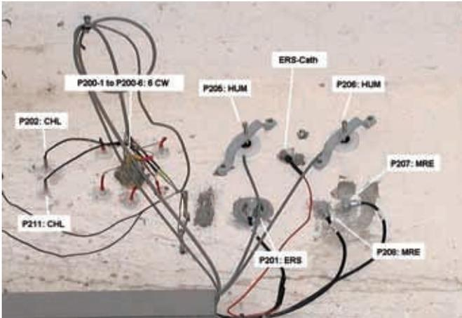
Group of sensors measuring deterioration on concrete structure.
